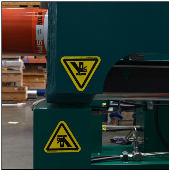
FIGURE 1-3. REAR CLAMP BOX AND FRAME LABEL LOCATIONS
