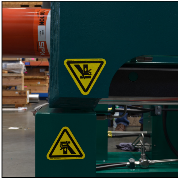
FIGURE 1-3. REAR CLAMP BOX AND FRAME LABEL LOCATIONS
