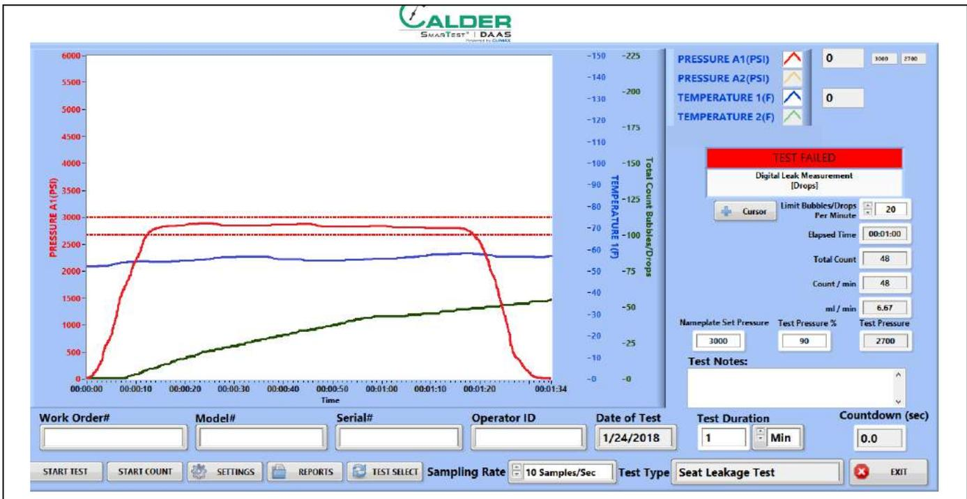
FIGURE 4-21. SEAT LEAKAGE FAIL EXAMPLE
