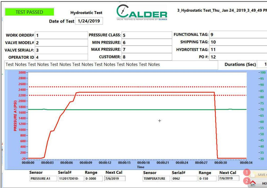
FIGURE 4-7. HYDROSTATIC REPORT INPUT SCREEN
