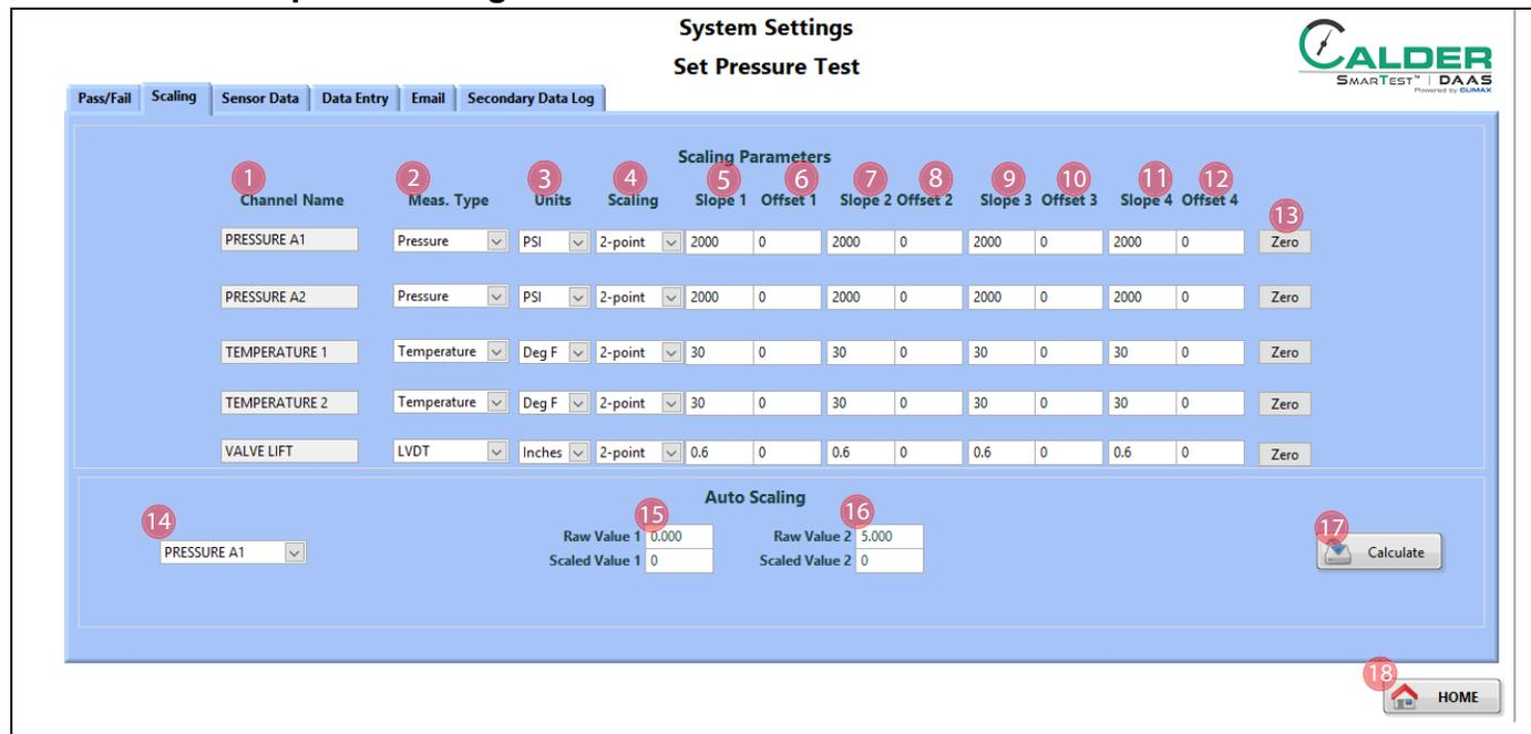
FIGURE 3-7. TWO-POINT SCALING SCREEN
