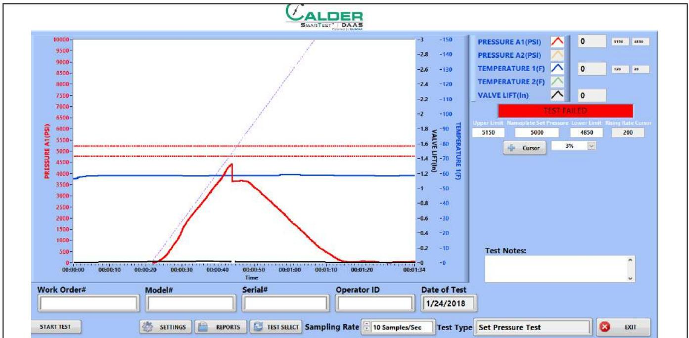
FIGURE 4-14. SET PRESSURE FAIL EXAMPLE
