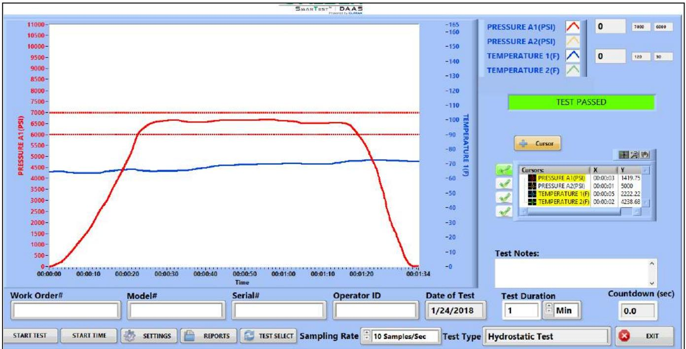
FIGURE 4-5. HYDROSTATIC TEST PASS EXAMPLE
