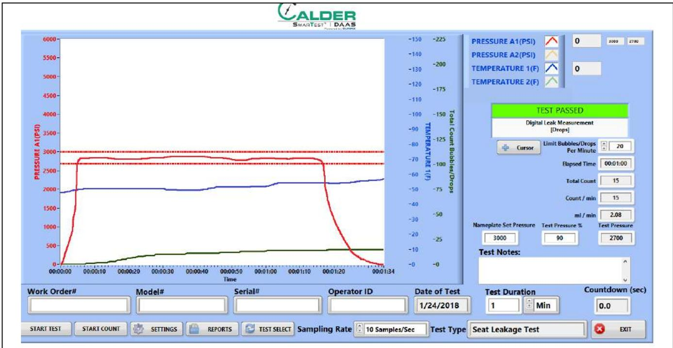
FIGURE 4-20. SEAT LEAKAGE PASS EXAMPLE
