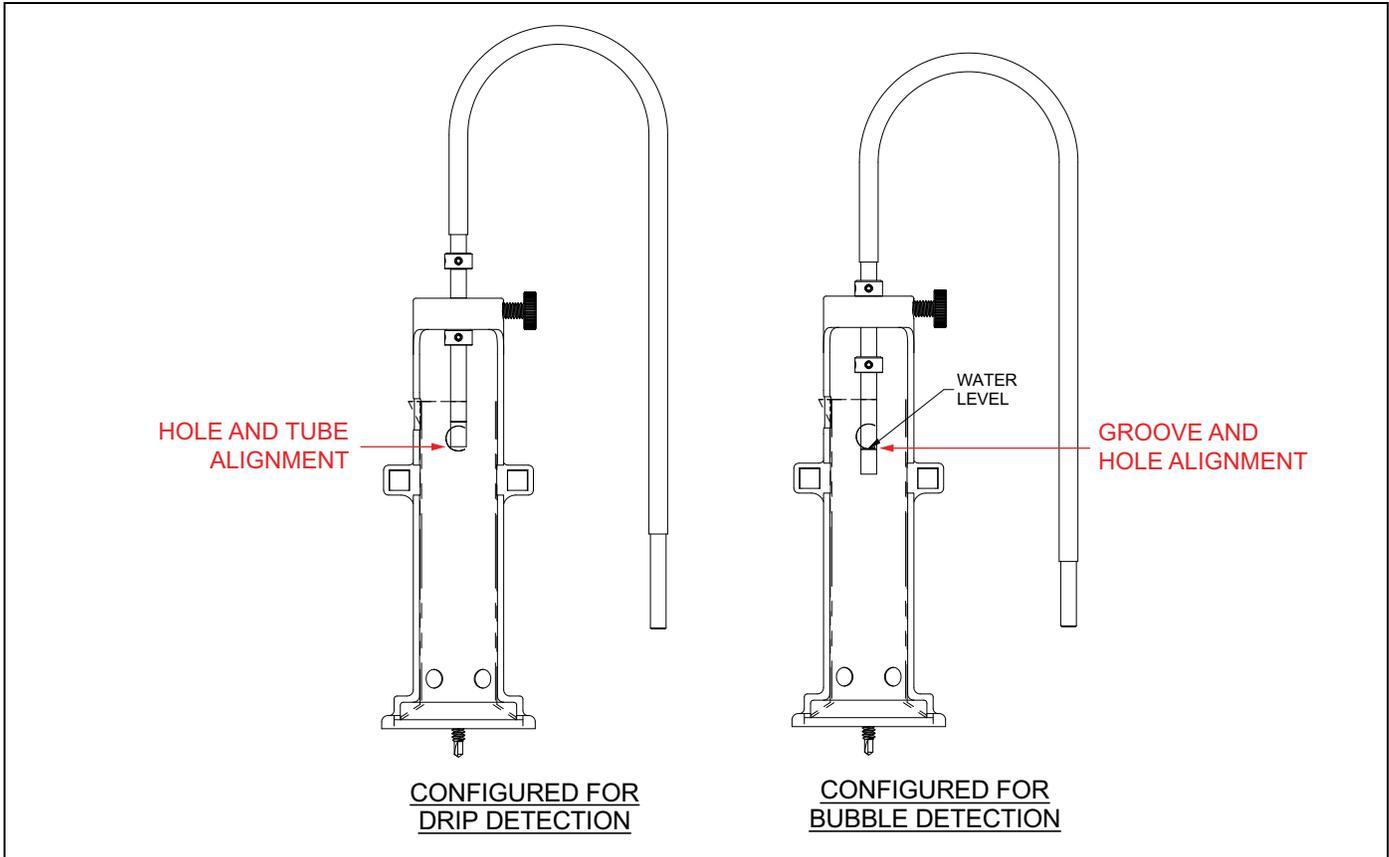
FIGURE 4-23. DIGITAL LEAKAGE MEASUREMENT SENSOR
