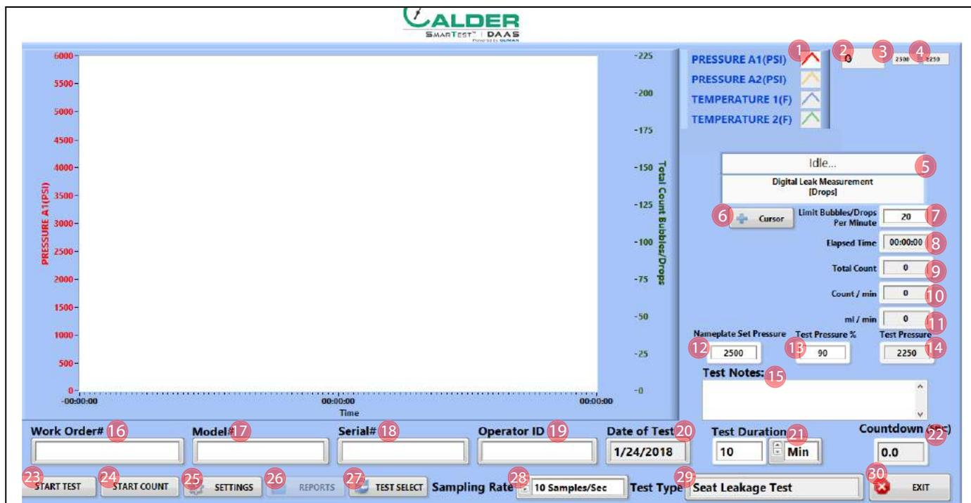
FIGURE 4-16. SEAT LEAKAGE TEST MAIN SCREEN
