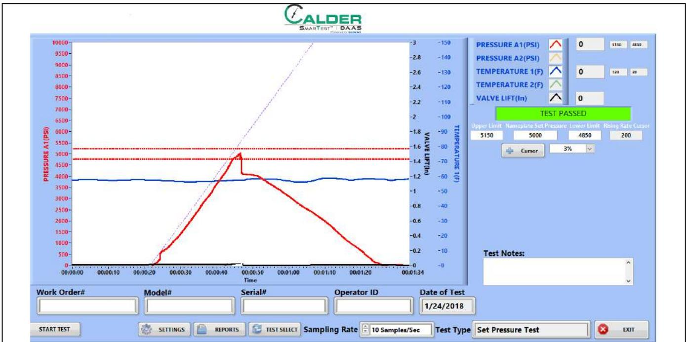
FIGURE 4-13. SET PRESSURE PASS EXAMPLE
